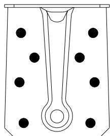
Figure D48-2: ABR7015 nail pattern
