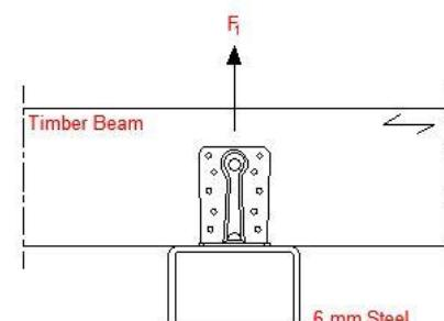
Table D11-7 1 angle brackets ABR9020, beam to column
