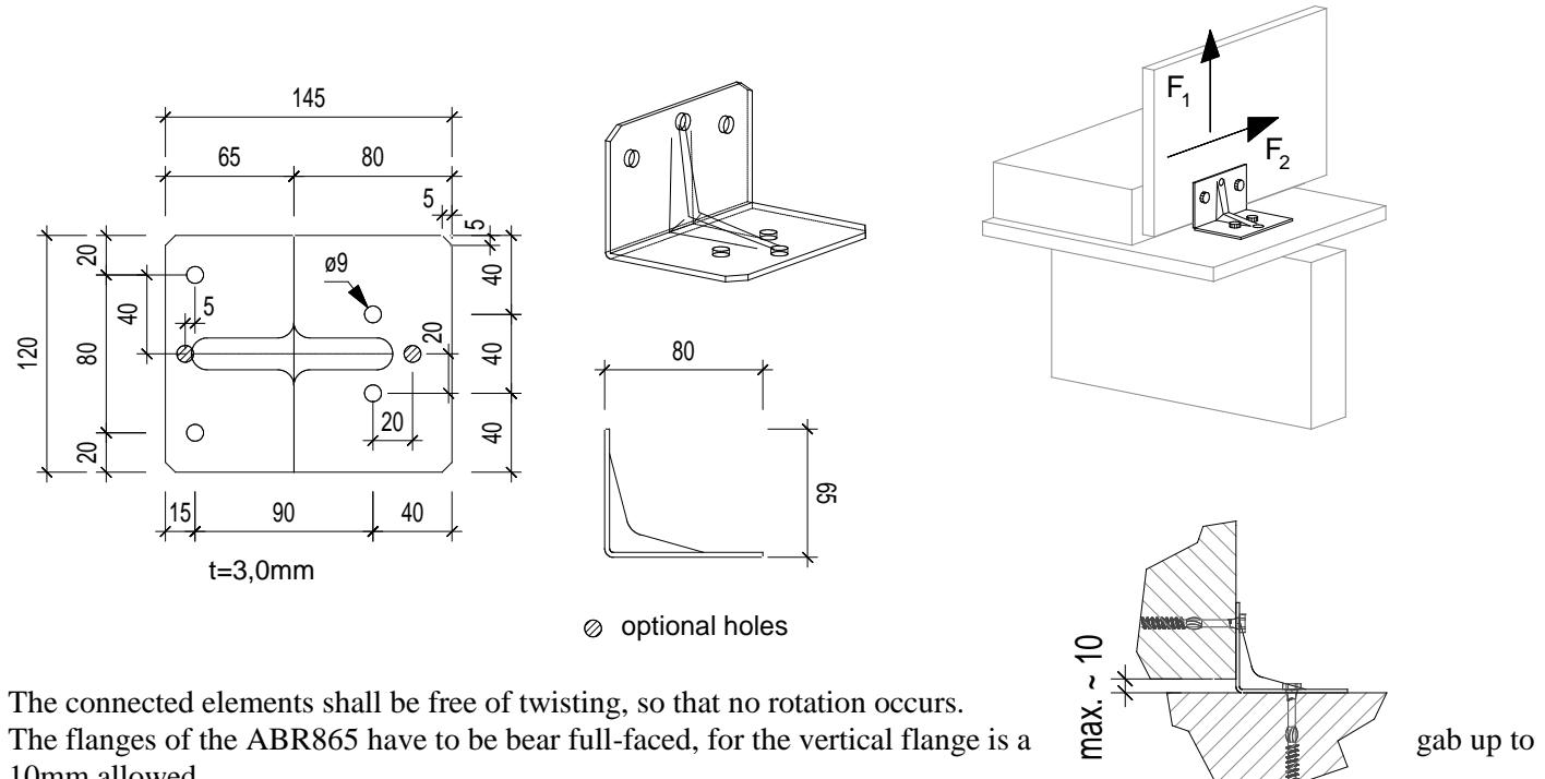
The connected elements shall be free of twisting, so that no rotation occurs.
