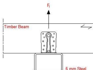
Table D47-6 1 angle brackets ABR10525, beam to column modified characteristic capacity per connection [kN]
