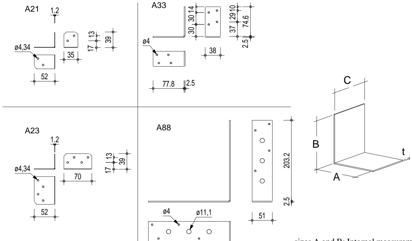
sizes A and B: Internal measurements
