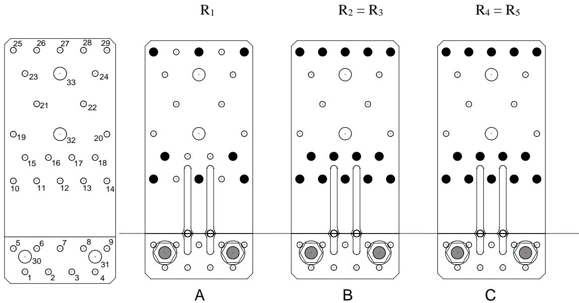
Figure D27-3 : ABR170 and ABR220 Nails patterns – Configuration A, B and C
