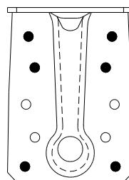
Beam to steel (6 mm S355) connection
