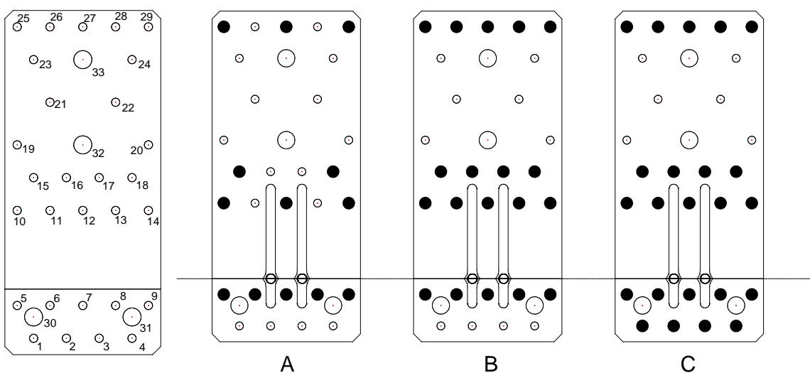
Figure D27-2 : ABR170 and ABR220 Nails patterns – Configuration A, B and C
