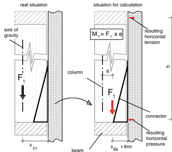
Generally the brackets shall be calculated with a lever arm of  $F_1$  of  $a_{F1} = (a_{dia} + 8\text{mm})$
