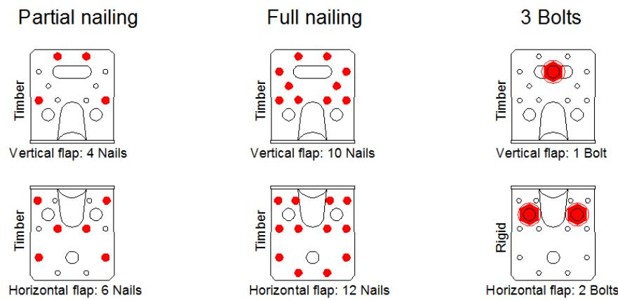
**Table D56-2: Characteristic capacity beam to beam – two Angle Brackets**
