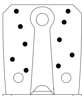
Beam to steel (6 mm S355) connection
