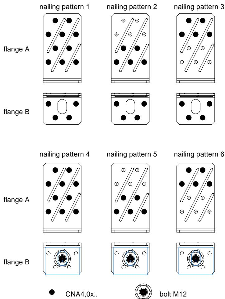
**Table D59-2: Characteristic capacity 1 Angle Bracket F<sub>1</sub>**
