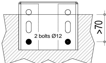
For the nail/bolt pattern A and B, the bolts are positioned with a sufficient distance to any border. The other nail/bolt patterns are for anchorage which has a minimum of 70 mm distance to the border of the concrete.
